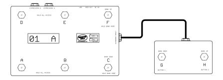
NOTE: The DMC-7D controller is identical to the DMC-6D except that the "H" button is located both on the expander switch jack and on the far right button of the controller.
