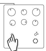
Power on the Meris pedal while holding the LED button over the left rootswitch. All of the Meris LEDs will blink three times to indicate that it is now in setup mode.
