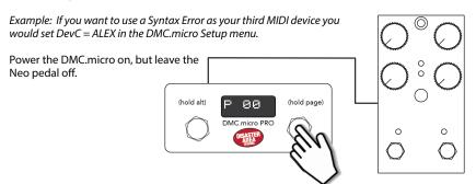
Hold and release the right footswitch on the DMC.micro until the device mode that you want to use is showing.
