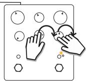
Rotate the lower right knob fully CLOCKWISE to set the EXP jack to MIDI. The far right small LED will light to indicate MIDI mode.
