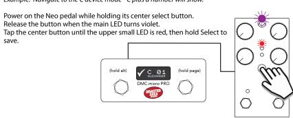
Power the Neo pedal off and back on, again holding the center button until the upper LED turns violet.
