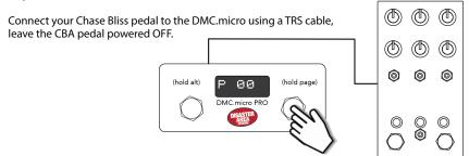
Hold and release the right footswitch on the DMC.micro until the device mode that you want to use is showing. As an example, we'll configure a Chase Bliss MOOD pedal as DevA.
