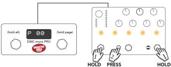
Enter the Advanced Configuration mode on the Empress pedal by holding the Select and Bypass footswitches, then pressing the Save button. The preset LEDs on the Empress pedal will blink yellow twice to indicate that you are in Advanced Configuration Mode.
