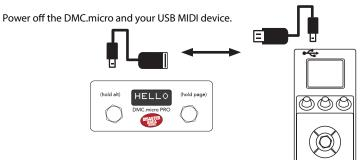
Plug the gHOST Adapter Cable into the USB port of the DMC.micro.
