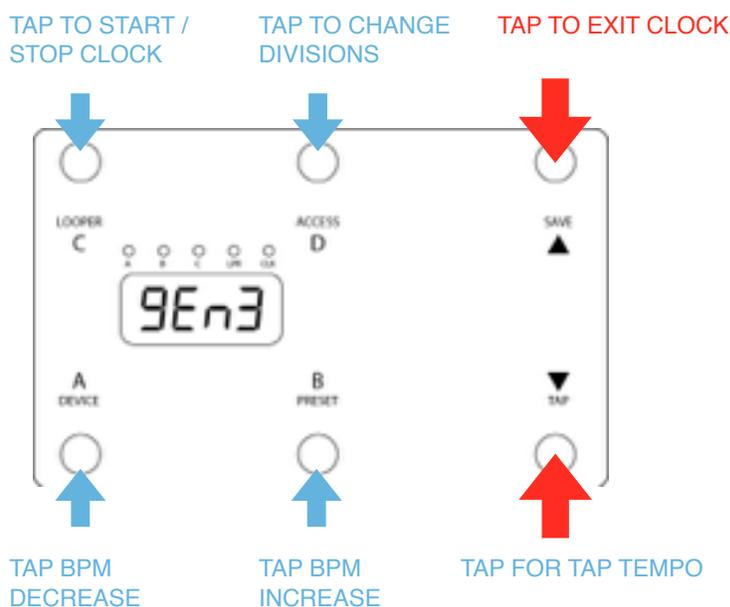
In the Setup Menu, there are four options for Tap and Clock Mode, each with different levels of functionality so that the user can decide the type of tempo control.
