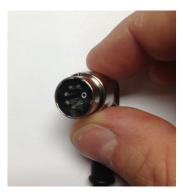
Gently rotate the pin sleeve until the pins face the desired direction.
