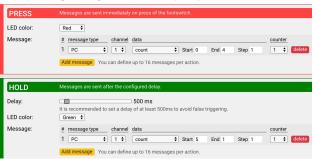
Step up through a range of values on tap, send the current value on hold - useful for Chase Bliss or Red Panda for saving presets
