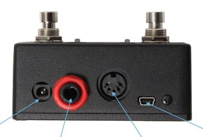
DC Power: 9V, 64mA minimum MultiJack: Connects to expression pedal, foot switch, MIDI, tap tempo, and more MIDI Port: Standard MIDI OUT on pins 4&5 MIDI INPUT on pins 1&3 USB Mini-B USB MIDI for computer or iPad, USB HOST for other USB devices
